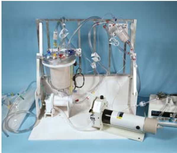
Air-transportable perfusion equipment designed around a hard-shell reservoir by perfusionist Melody Maxim for Suspended Animation.
